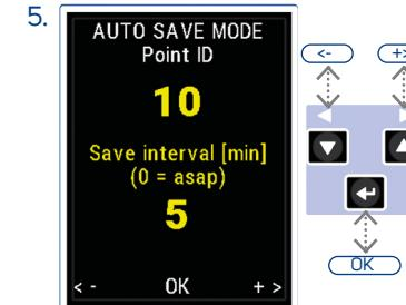
Select the time interval for data saving (1-60 minutes, 0 is for the maximum speed of data storage)
