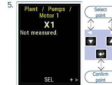
Use the Arrow buttons to switch between the points in route
