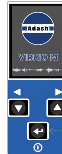
Press the Enter button to switch on the device
