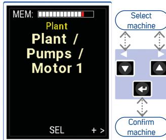
Use the Arrow buttons to switch between the machines in route
