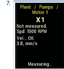
Measurement progress can be seen on the screen
